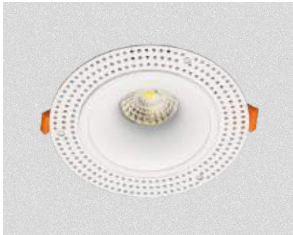
TRF5-W Fixed Mounting Ring IP Rating: IP20/IP44 Casting Color : White / Black / Customized Cut out Ø100mm
